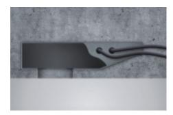
The trimless installation in cast concrete ceilings can be realised using specially developed cast-in housings. The use of a variable core element means this is also possible with bare concrete ceilings.
