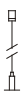
Wire-rope suspension, system B 1762.111 wire rope L= 1000mm 1762.112 wire rope L= 2000mm
