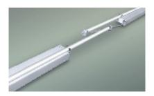
With a width of just 52mm this system luminaire is designed for particularly narrow installation scenarios. The lamps are arranged in an overlapping formation. The clip fixing for the lamps facilitates maintenance for inaccessible light shelves.
