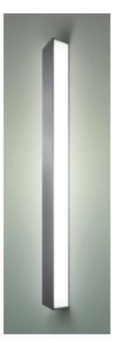
Wall Luminaire, Indirect A single luminaire. Aluminium profile luminaire in powdercoated silver C3 or any RAL colour. Lateral light output covered with satinized opal silk acrylic diffuser. Luminaire equipped for T5 HE or HO fluorescent lamps with integrated electronic control gear. 3-pole terminal block for through-wiring. Easy wall assembly due to accessible installation housing.
