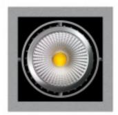
Cardanic LED downlights Recessed-mounted housing made of sheet-steel, with slender frame for installation in sawn ceiling cut-outs. Powdercoated surface. Equipped with high-power LED arrays. With aluminium reflector, silver, polished and individually anodized, optionally available with different beam characteristics. The luminaires are supplied complete with electronic control gear.
